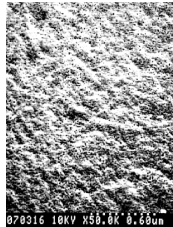
Pore size: 0.01 micrometer
