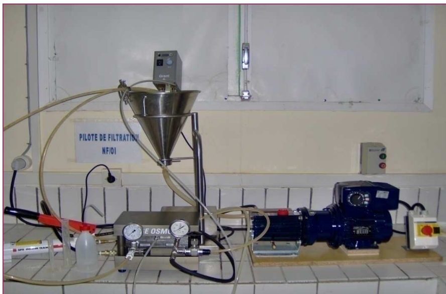
Figure 20 : Picture of the experimental set up used for salt mixture and real water experiments (Module SEPA CFII)
