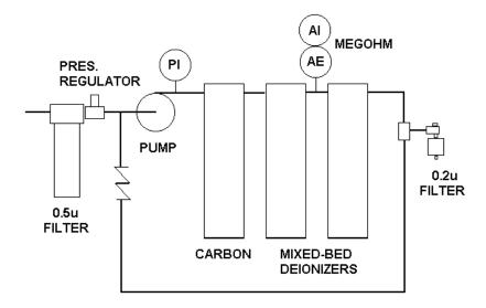
FIG. 1 - LABORATORY TYPE I REAGENT GRADE SYSTEM
