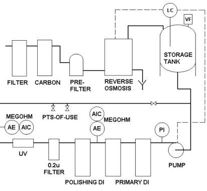
FIG.2 - CENTRAL WATER SYSTEM ASTM TYPE I
