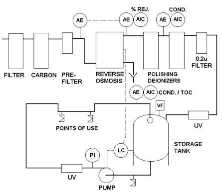
FIG. 3 - USP PURIFIED WATER SYSTEM
