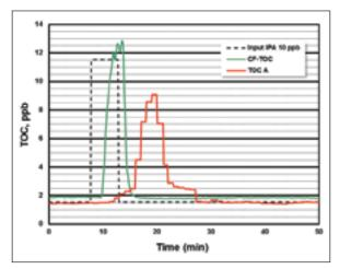
Figure 1: IPA response curves. CF TOC vs TOC A.
