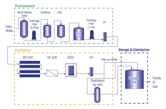
Schematic of a Pharmaceutical Water Preparation System
