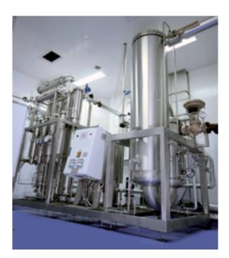
tem from the incoming feedwater to pretreatment to purification to final distribution, in order to measure and control water production and quality. Some of these in-process measurements include conductivity, TOC, dissolved ozone, pH, ORP, silica, turbidity, flow rate, % rejection, tank level, temperature, and pressure.
