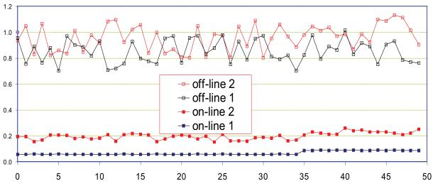
Fig. 1: Comparison of on-line and off-line conductivity measurements of two high purity water samples
