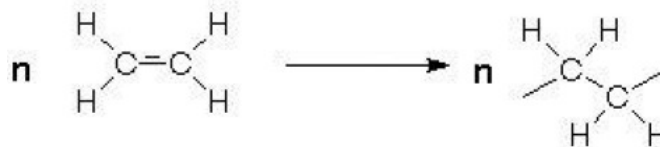
Figure 3-10 Typical polymerisation reaction by opening double bond
