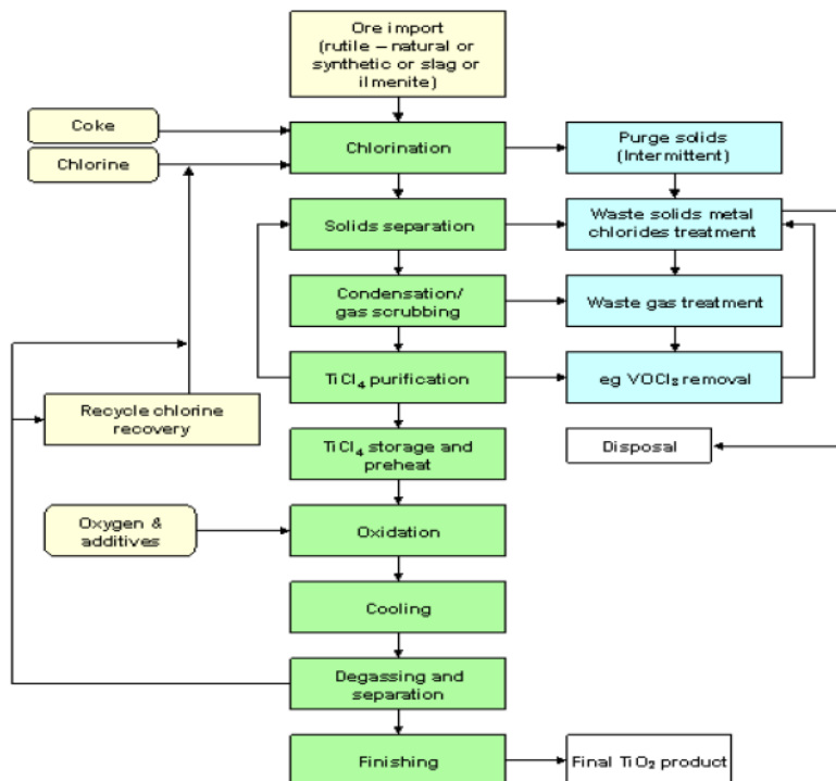
Figure 3-8 Process flow for manufacturing of \text{TiO}_2 (Chloride process) [20, CEFIC-TDMA, 2004]
